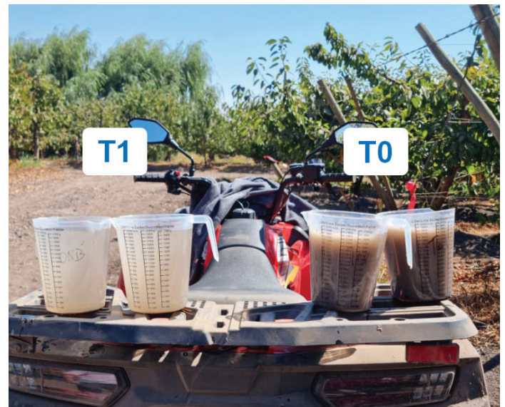
Figure 1: Comparison of sediments in irrigation water T0 = Control, T1 = Treatment with nanobubbles
