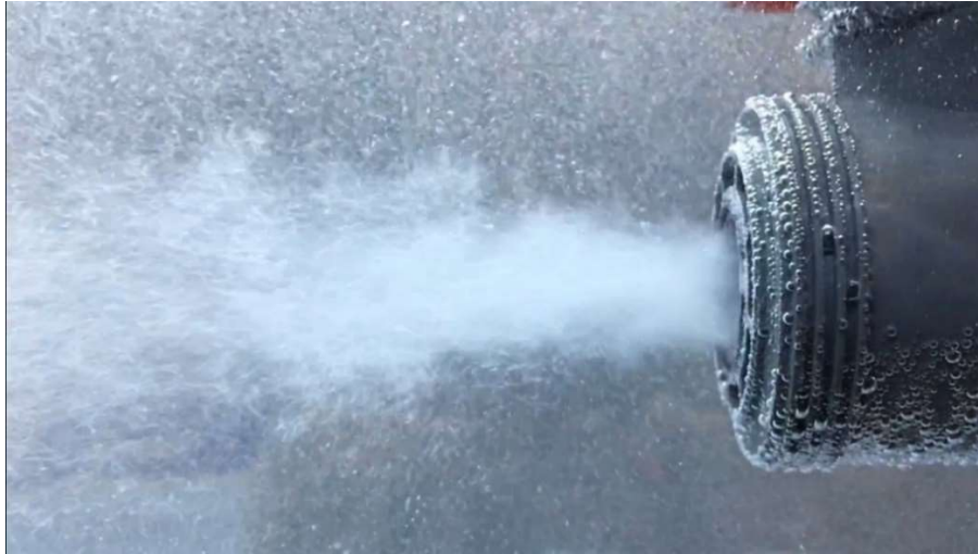
Figure 10: Bubble pattern for a proper installation
