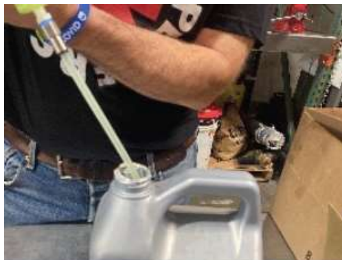
Figure 20: Filling syringe with cleaning solution
