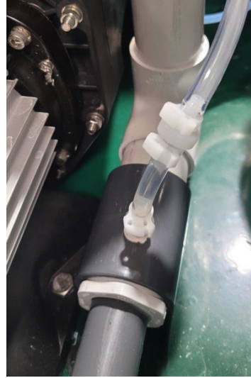
Figure 12. Clamp Disconnected and CIP Tube Inserted into Nanobubble Generator
