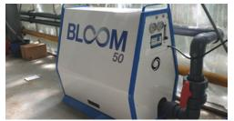
The Bloom nanobubble generator quietly and efficiently supersaturates irrigation water with dissolved oxygen.
